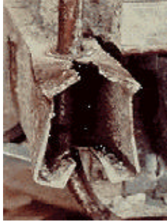
Figure 1 – Failed beam of Kansas City Hyatt Regency walkway
